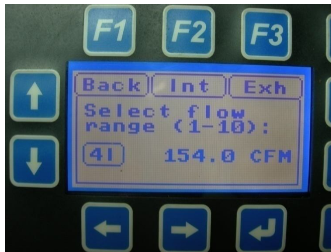
Figure 3.19: Orifice range flow at the test setup
