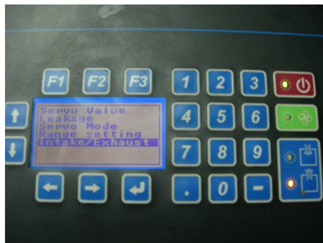
Figure 3.20: Setting the exhaust orifice flow at the flowbench display screen
