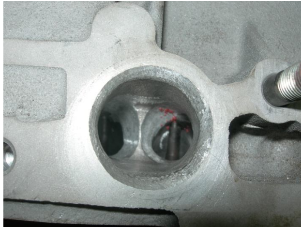
Figure 3.6: Toyota cylinder head after porting process
