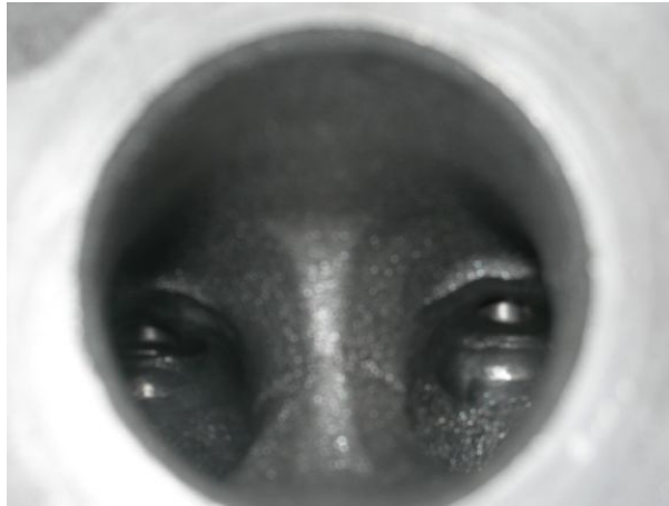
Figure 3.4: Valve guide removed in Toyota cylinder head
