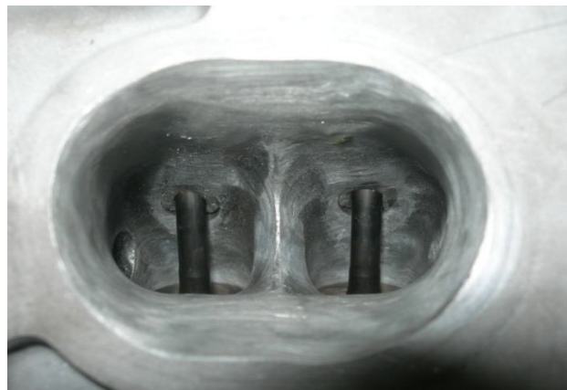
Figure 3.7: Proton cylinder head after porting and polishing process
