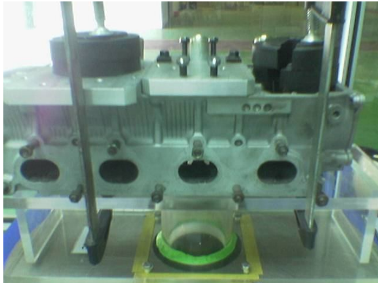
Figure 3.15: Cylinder head attached to the adapter by clamping with G-clamp
