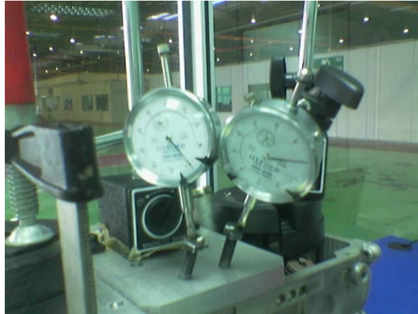
Figure 3.16: Dial gauge indicator attached to the thread screw
