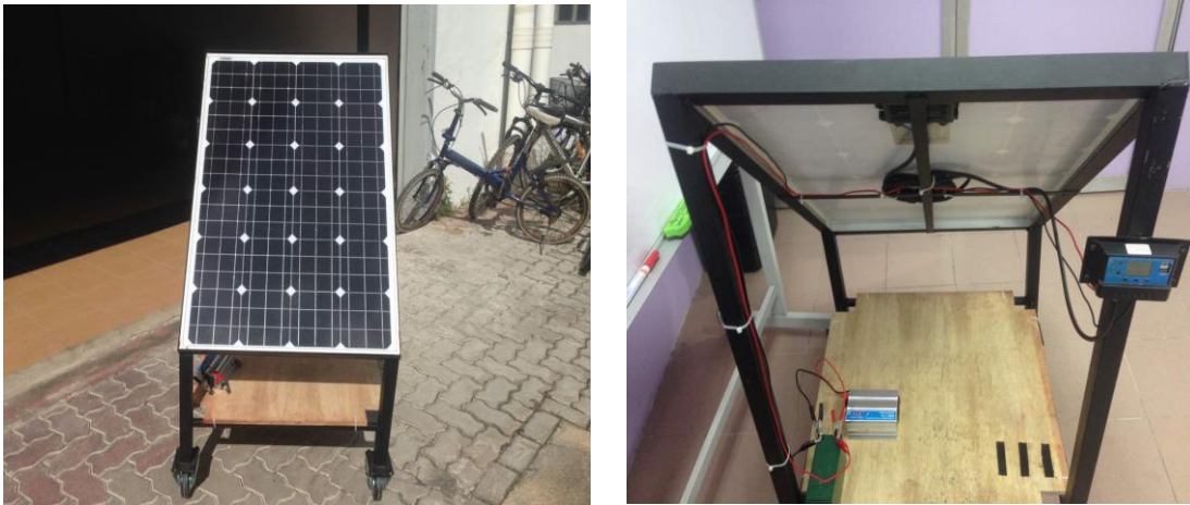
Figure 9. 90W of solar charging station
