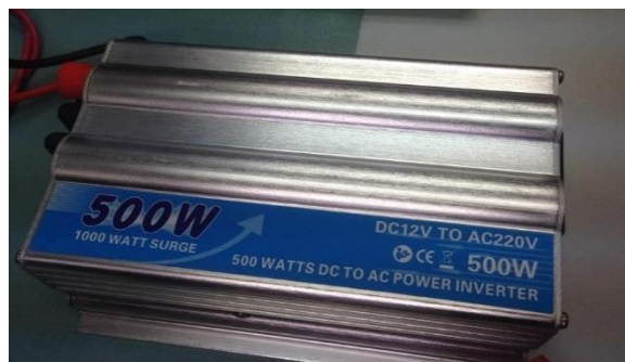
Figure 8. 500W of solar inverter
