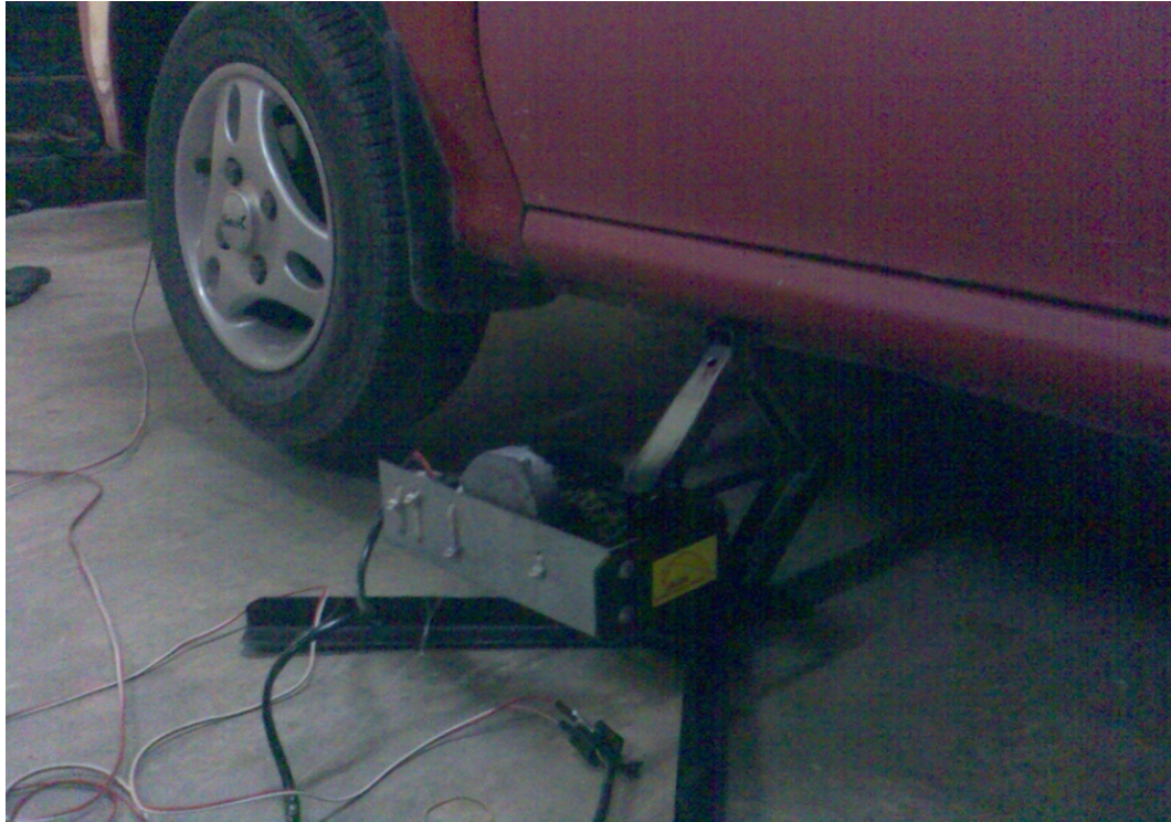
Final test after re-fabricated the frame holder
