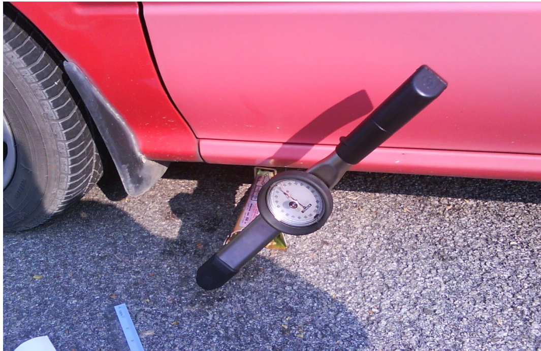
Using torque wrench to observed the torque needed
