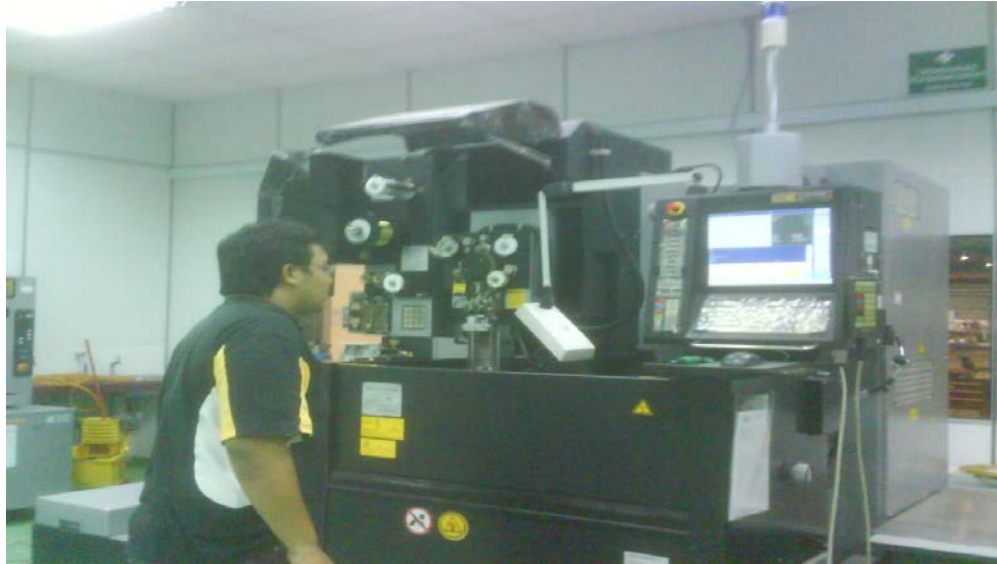
Programming the gears design into wire EDM machine
