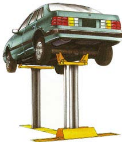
Figure 2.7: A double post in ground lift
