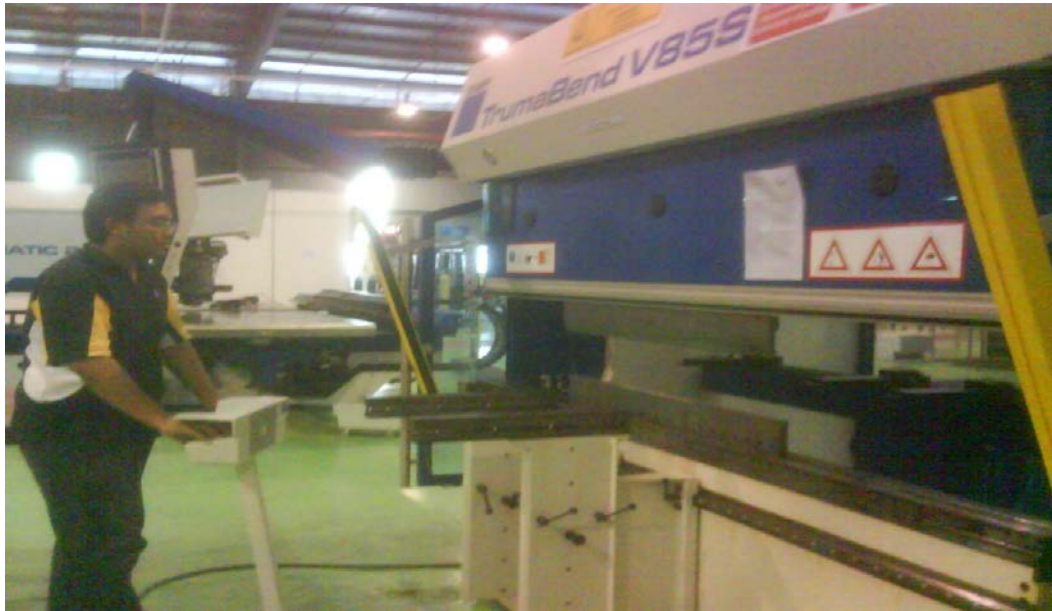
Using bending machine to bend the cover for the gearing system
