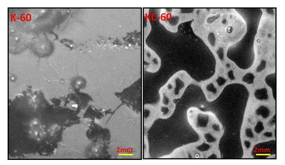
Fig. 2. SEM images of synthesised bioplastics.
