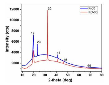
Fig. 3. X-ray diffractogram of synthesised bioplastics.
