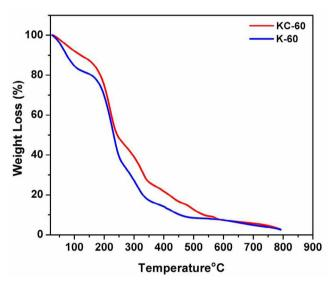
Fig. 4. TGA graph of synthesised bioplastics.
