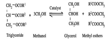
Transesterification reaction will take part in this process to produce the high quality biofuel. Finally, the product of jatropha oil can be use as a biodiesel in transportations and vehicles.
