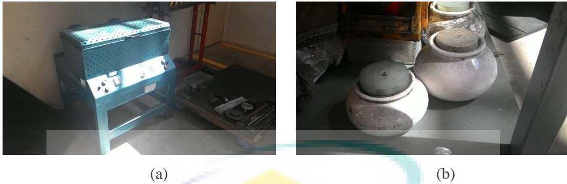
Figure 3.5 Material preparation for treatment a) Fast Mills Machine b) Material container during milling process
