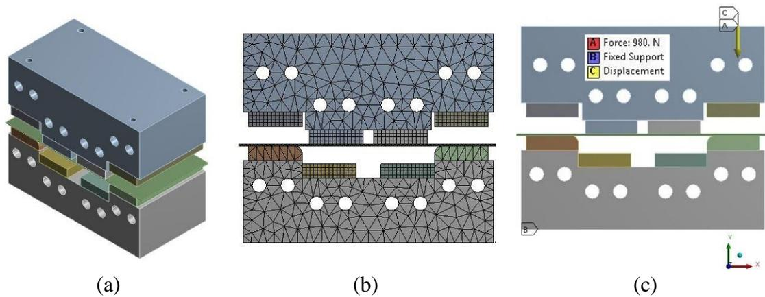
Figure 4. Geometry model in ANSYS Workbench (a) Geometry model generated in ANSYS, (b) Meshing condition of model, (c) Loading and boundary condition.
