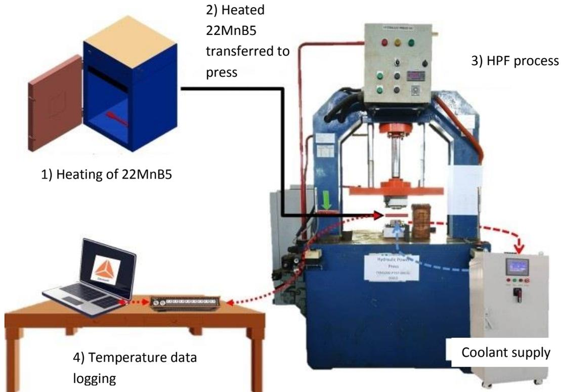
Figure 1. Experimental setup of boron steel 22MnB5 test.
