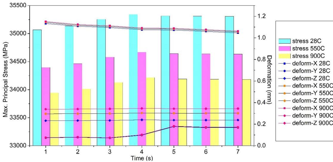
Figure 11. Graph of principal stress and deformation against the HPF process duration.
