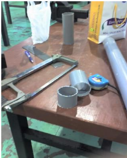
Figure 3.4: Cutting Of PVC Pipe
