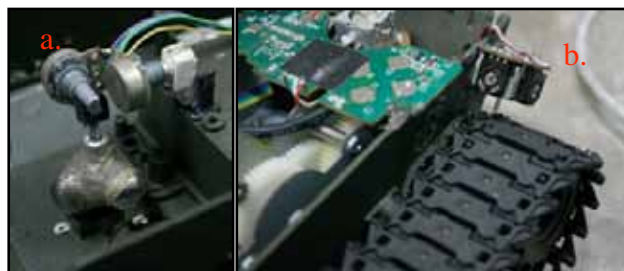
Fig.2.JOMS module(a) Pendulum as inclinometer. (b) Potentiometer as rotary encoder.
