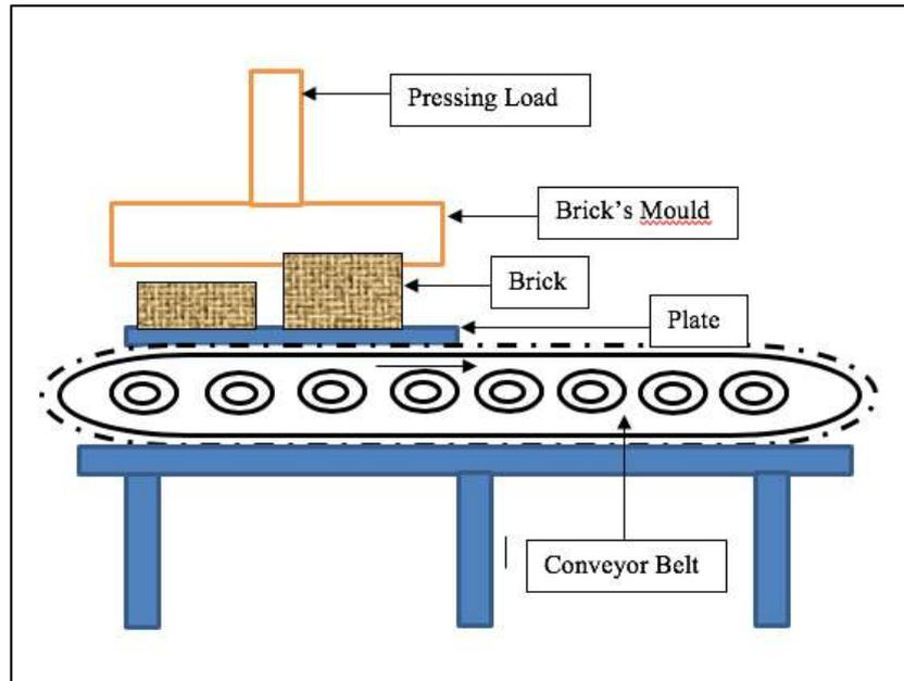
Figure 1. Illustration on how thickness affects the surfacing of bricks.
