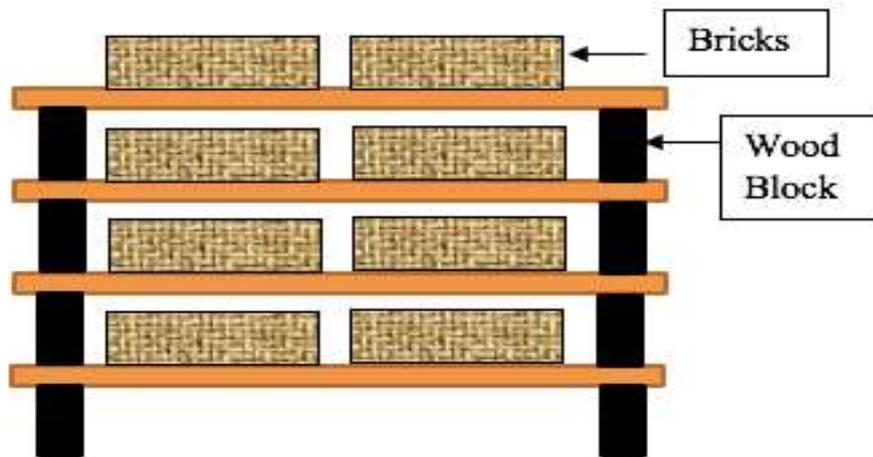
Figure 3. Illustration of transportation and drying with wood block
