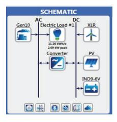
Fig 1. PV-Wind-Diesel Power System Configuration.
