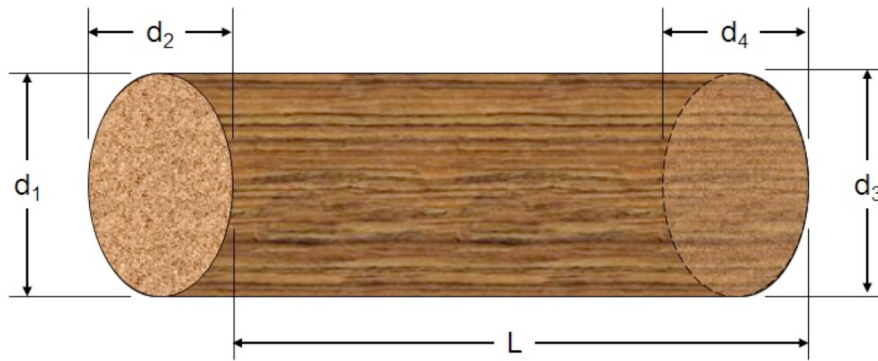
Figure 3 Geometrical measurements of Smalian's formula
