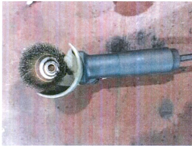
Figure 3.13: Bowl-type wire wheel wire brush used to remove rust
