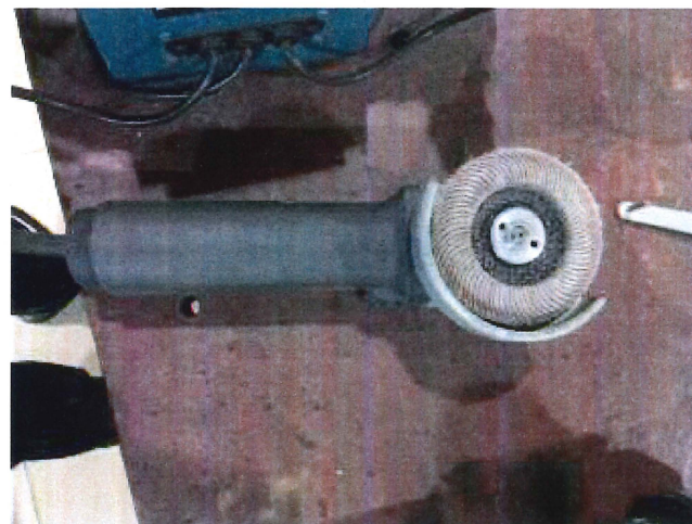
Figure 3.14: Tools to remove welding wear
