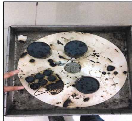
Bitumen Penetration Test
