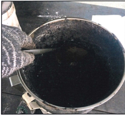
Aggregates and bitumen manually mixed
