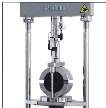
Figure 3.3: Marshall test setup
