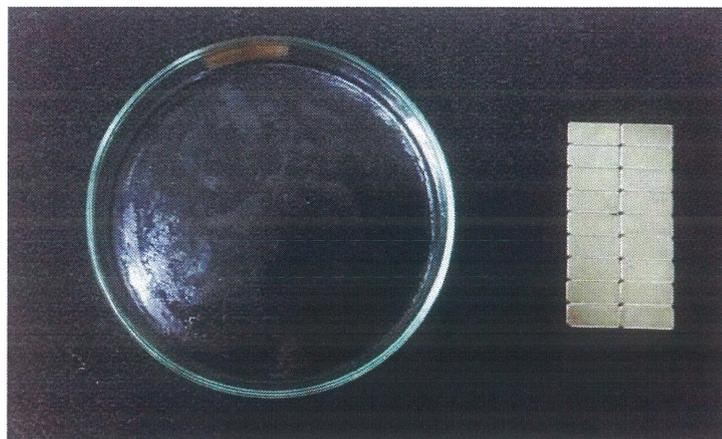
Apparatus set-up for Meissner Effect Test. The needed apparatus are strong magnet (neodymium magnet) to form a plane or trail at least, petri dish and liquid nitrogen. The main purpose of doing this testing is to classify whether the sample having superconducting behavior or negative. This Meissner Effect occur when any type of superconductor obtained its transition temperature and completely repel the magnetic field.
