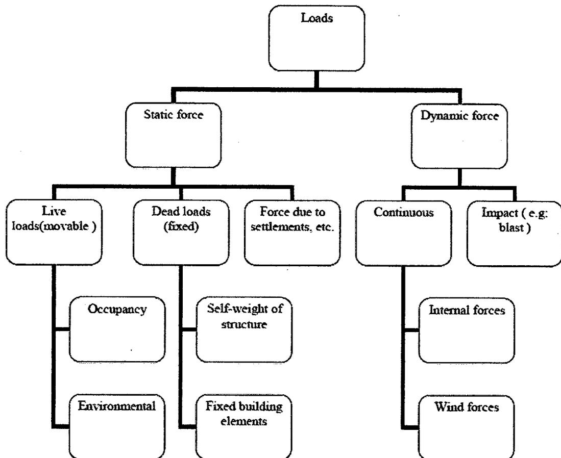
**Figure 2.2** Typical types of loading condition
