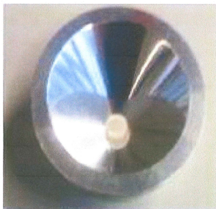
Figure 2.3 Close view of conical mirror.
