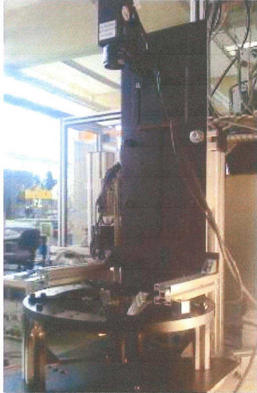
Figure 2.4 Matrix camera with multiple flat mirrors system.
