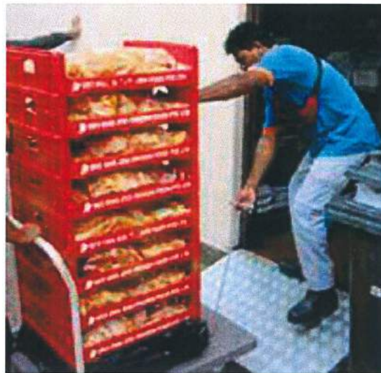
Figure 4.1: Trays with proper handholds for better grip
