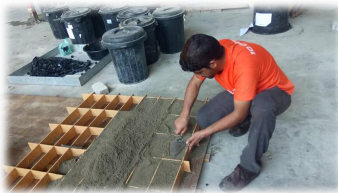
Photo-2: Oiling, casting and compacting Process
