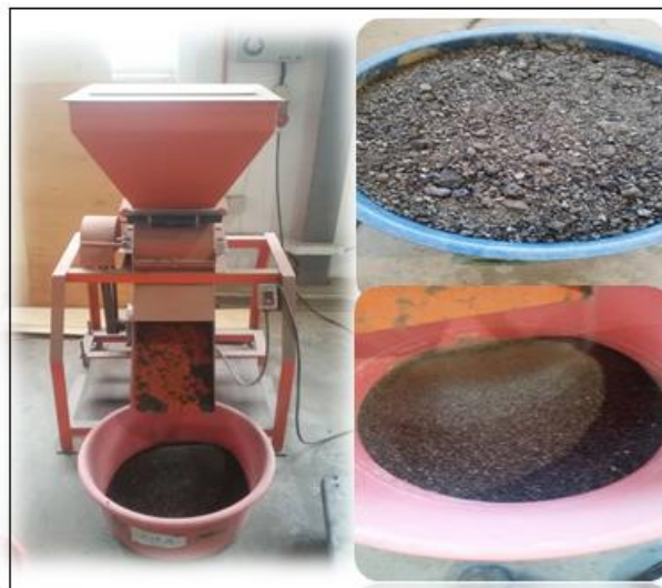
Fig-1: Grinding Bottom Ash
