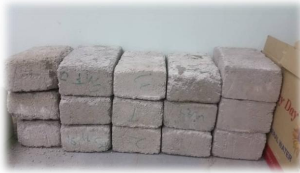
Fig-2: Air Curing of bricks
