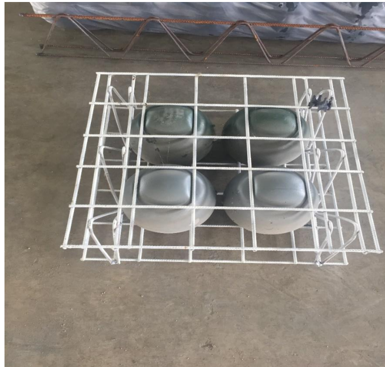
Figure 3.3 Small-scaled Bubble Deck sample
