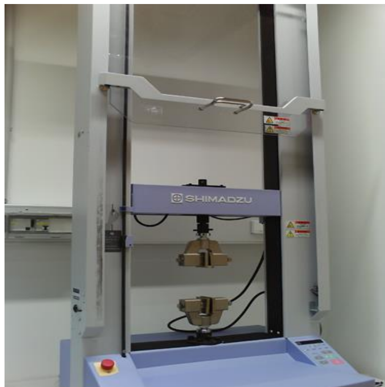
Figure 3.7 Universal tensile testing machine
