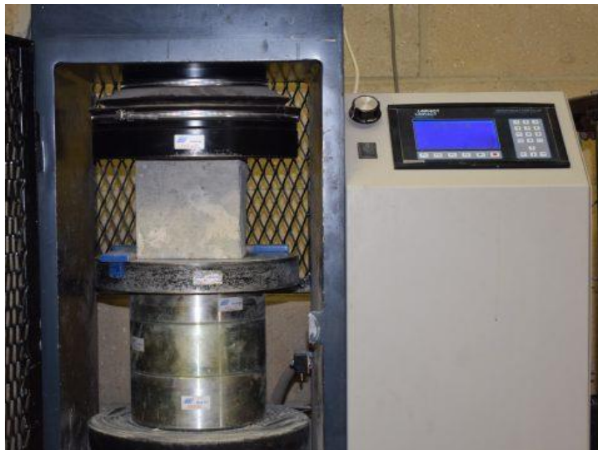
Figure 3.9 Concrete compression test
