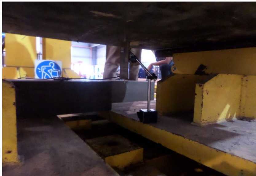
Figure 4.8 Set-up of LVDT
