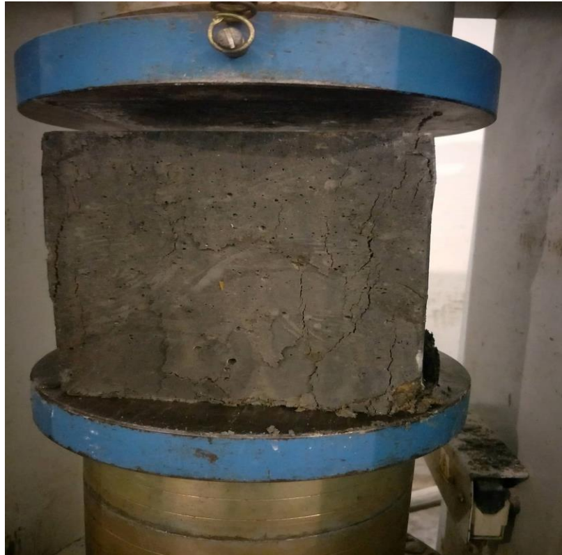
Figure 4.4 Failure of concrete cube specimen
