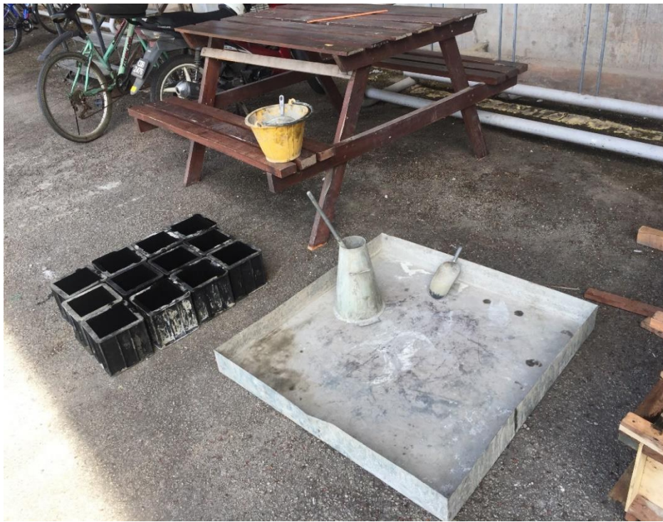
Figure 3.4 Preparation of slump test
