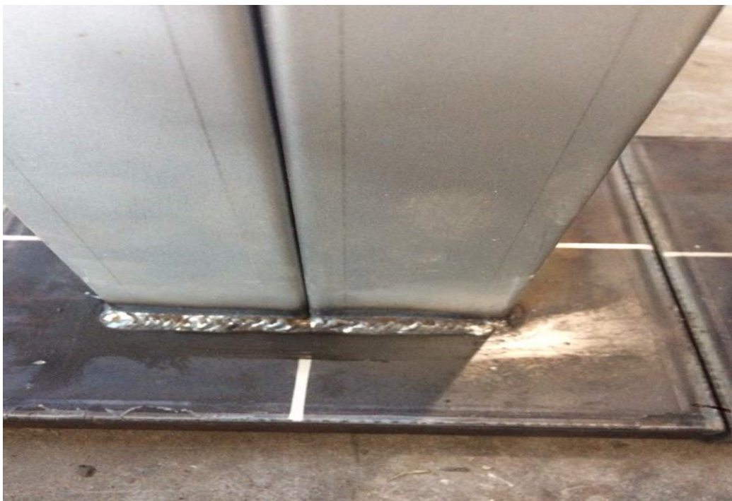
Figure 3.7 The Support Condition of the Specimen
