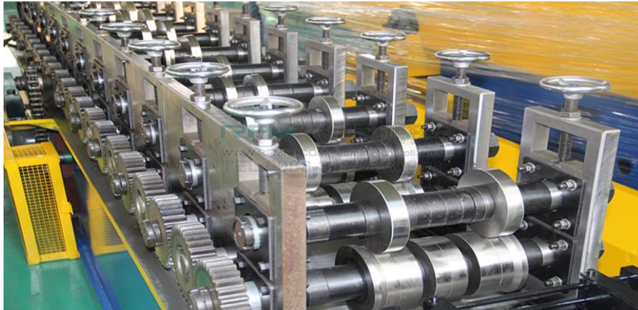
Figure 2.3 Cold Roll Forming Machine
