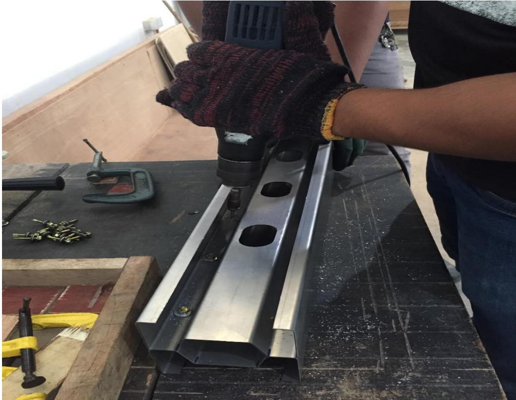
Figure 3.4 Drilling the Specimens to form Build-up Section
