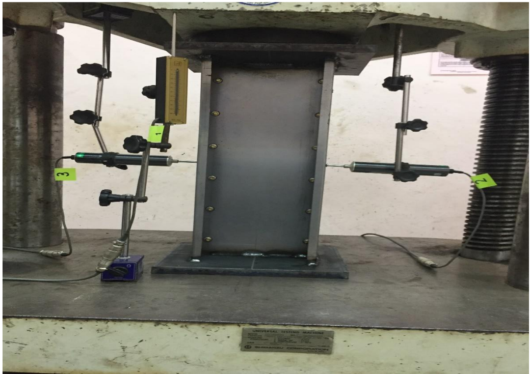
Figure 3.9 The Placement of Transducers and Specimens
