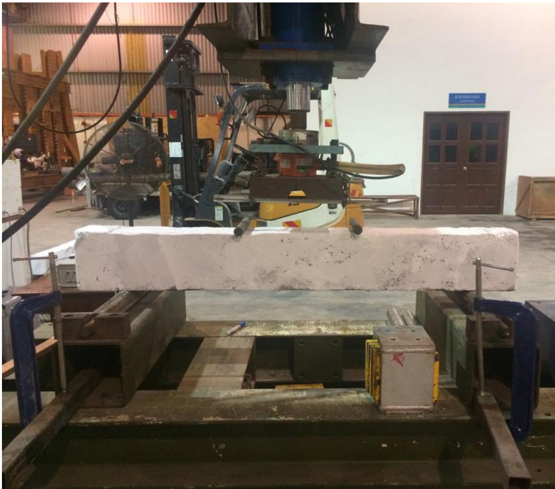
Figure 3.11 Testing Set Up of the Beam
