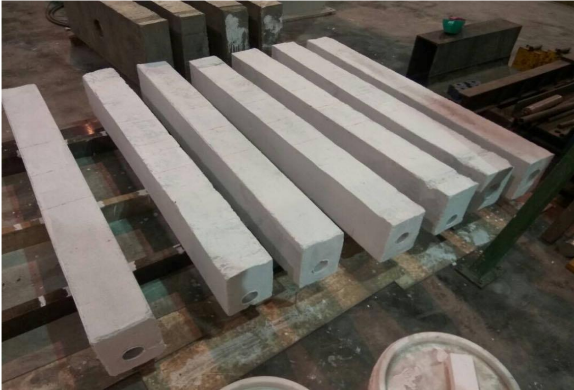
Figure 3.10 Painting of the beams
