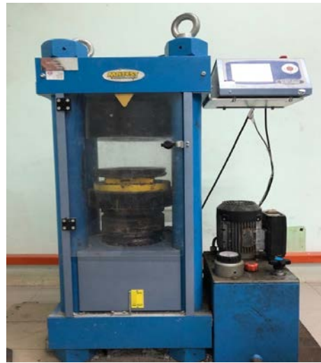
Figure 3.12 Compressive Strength Test Machine
