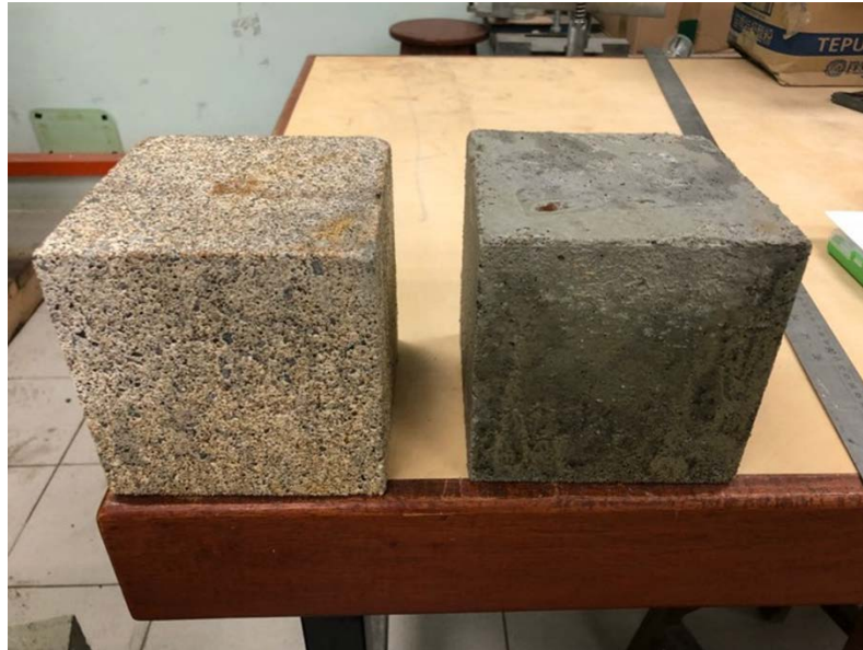
Figure 4.6 Cube specimens for 0FA 0ESP (left side) and 30FA 5ESP (right side) after immersed in acid solution for 90 days
