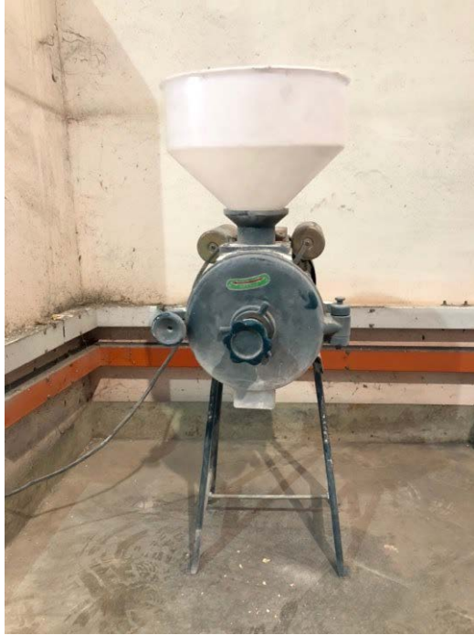
Figure 3.3 Grinding machine used to grind eggshell into powder form
