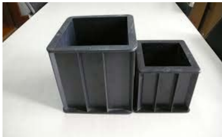
Figure 3.10 Plastic cube mould of size 100mm and 150mm
