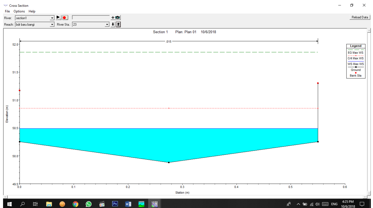
Figure 4.19 Cross Section CH23(2 YEARS ARI)
