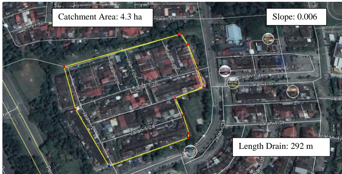
Figure 4.3 Details of Catchment Area
