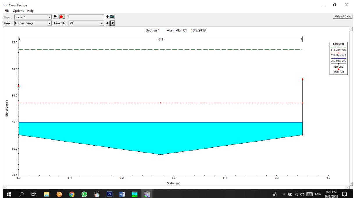
Figure 4.47 Cross Section CH23(5 YEARS ARI)
