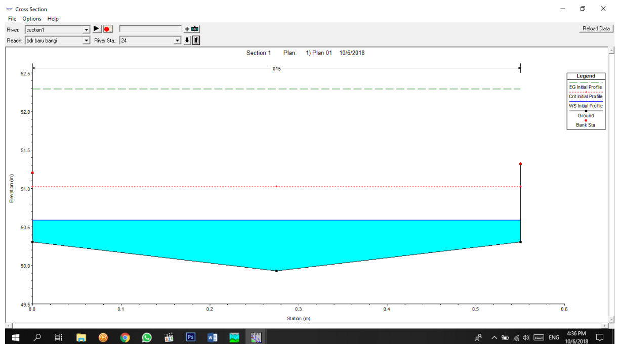
Figure 4.74 Cross Section CH24(10 YEARS ARI)
