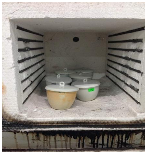
Figure 2.3 Furnace used in the organic content test
