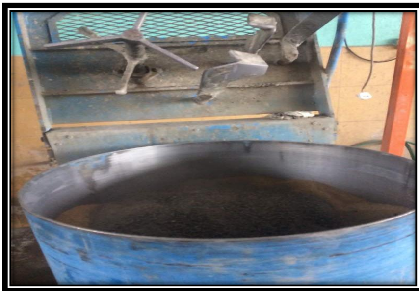
Figure 3.12 All weighted material mixed together into the mixer
