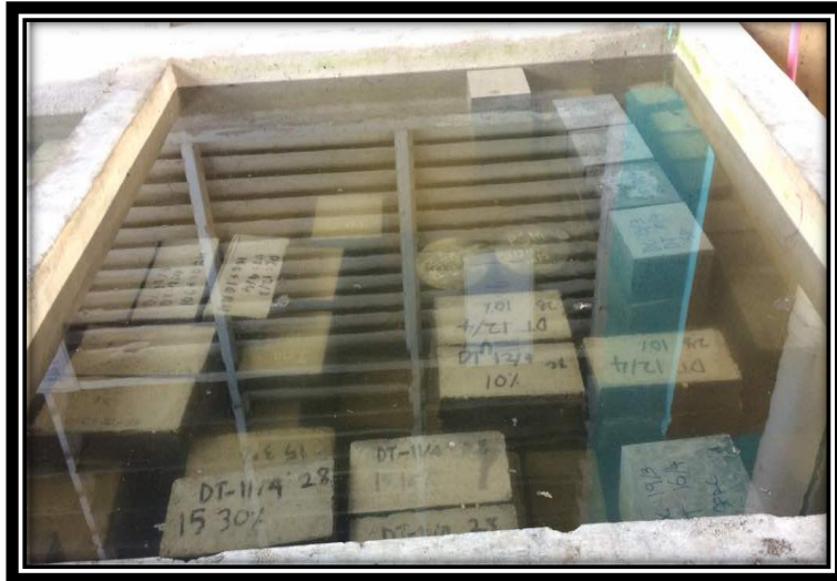
Figure 3.16 Water curing process
