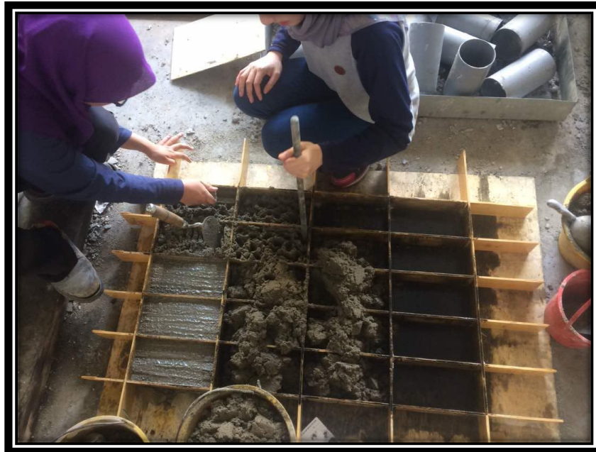
Figure 3.14 Process compaction of brick samples
