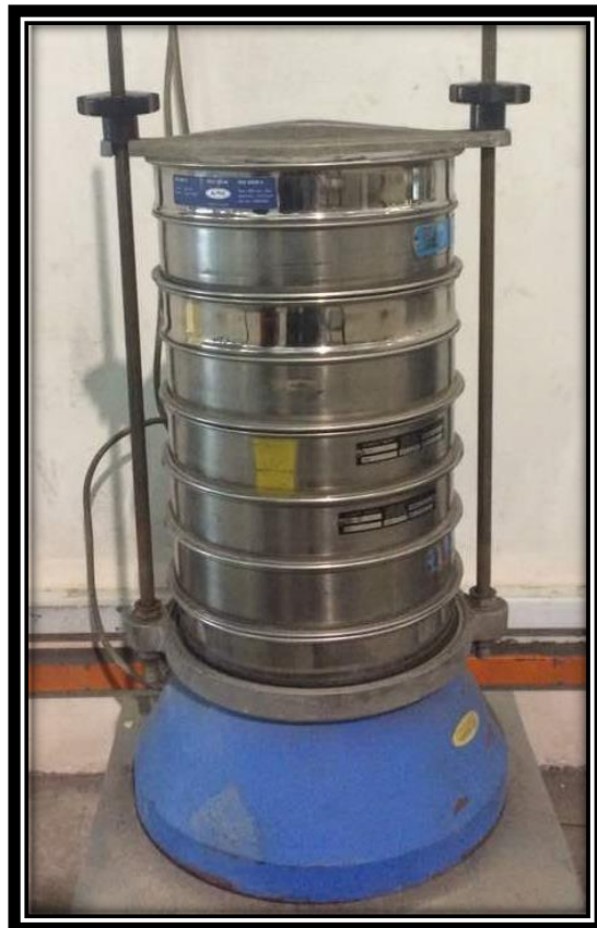
Figure 3.4 Sieve analysis process
