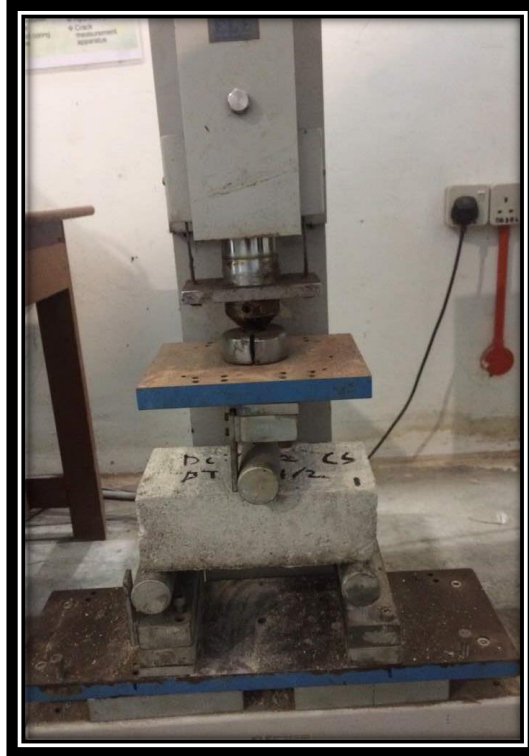
Figure 3.19 Flexural strength test
