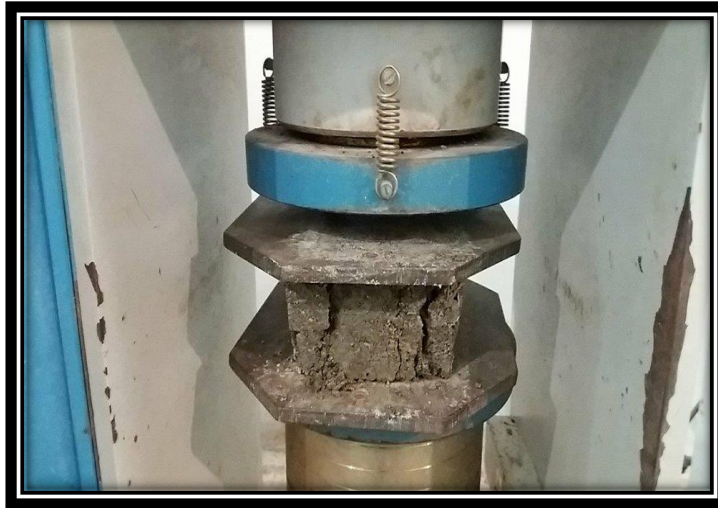
Figure 3.18 Sand brick condition after undergone compressive strength test
