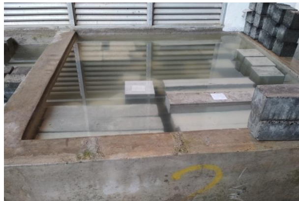
Figure 3.8: Process of water curing
