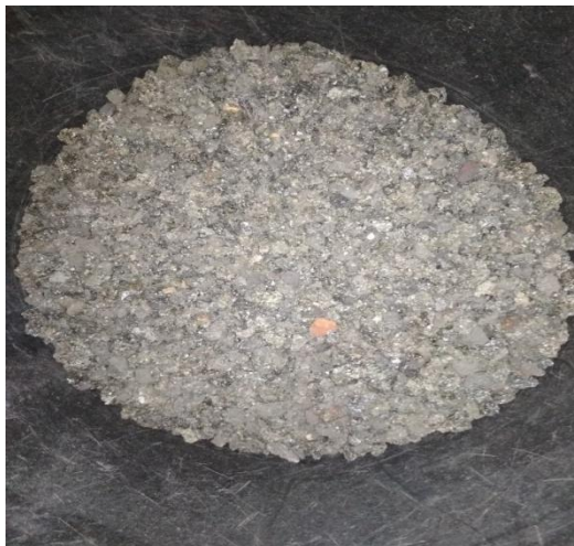
Figure 3.6: Palm oil clinker after pulverizing process
