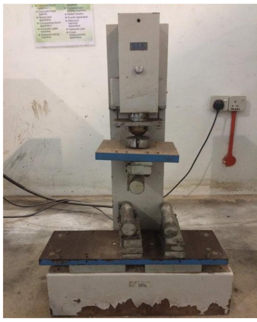
Figure 3.10: Flexural strength testing machine
