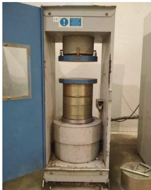
Figure 3.9: Compressive testing machine
