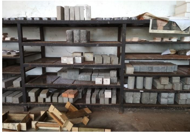
Figure 3.7: Process of air curing
