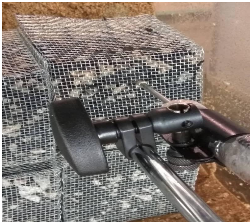
Figure 3.6 Digital transducer must be 90° angle with the wall
