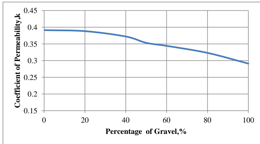
Figure 4.13 Coefficient of permeability against percentage of gravel
