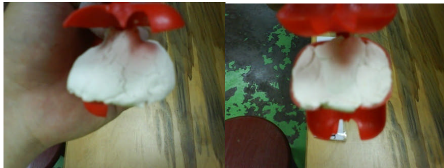
Figure 3.1.2.a & 3.1.2.b: Retrieving shape from existing Pelton
