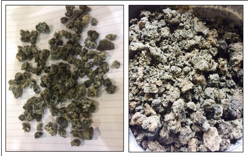
Figure 3.5 Palm Oil Boiler Stone (POBC).
