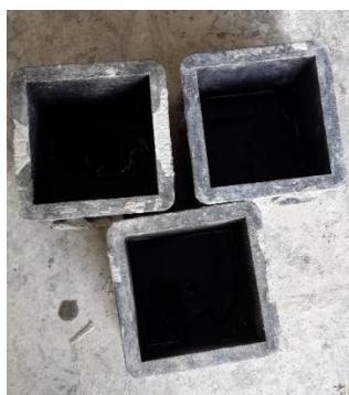
Figure 3.8: Steel mould (150mm X 150mm X 150mm)
