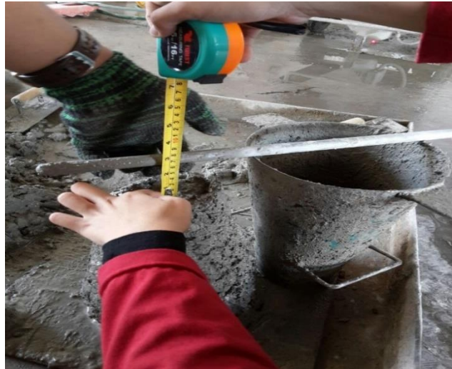
Figure 3.1: Slump test to measure the workability of a fresh concrete
