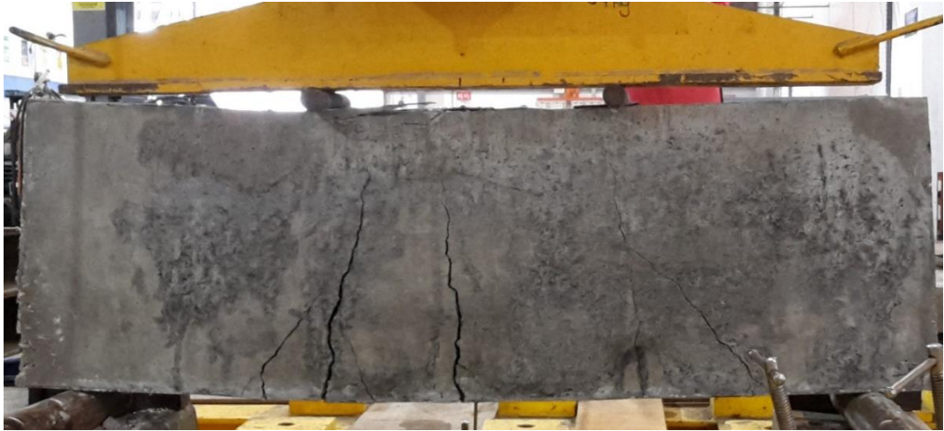
Figure 4.16: Cracking pattern for control beam without opening
