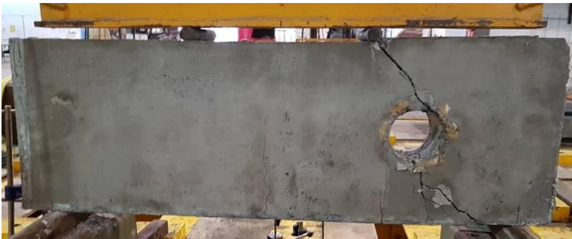
Figure 4.17: Cracking pattern for control beam contain 0% of hybrid fibre
