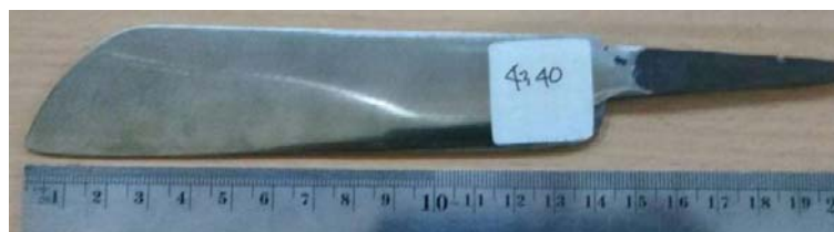
Figure 2 Steel knife 4340 manual forging results
