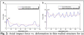
**Fig. 2:** Axial impact force vs. deformation in thin-walled structure for (a) hollow thin-walled structure and (b) foam-filled thin-walled structure.[15]
