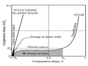
Fig. 1: Stress-strain curve of a foam
