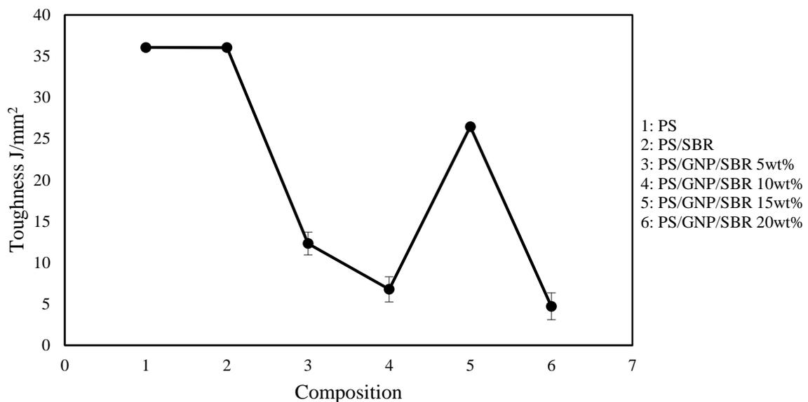
**Figure 3.** Impact resistance of SBR toughened PS/GNP nanocomposites at various contents of SBR.
