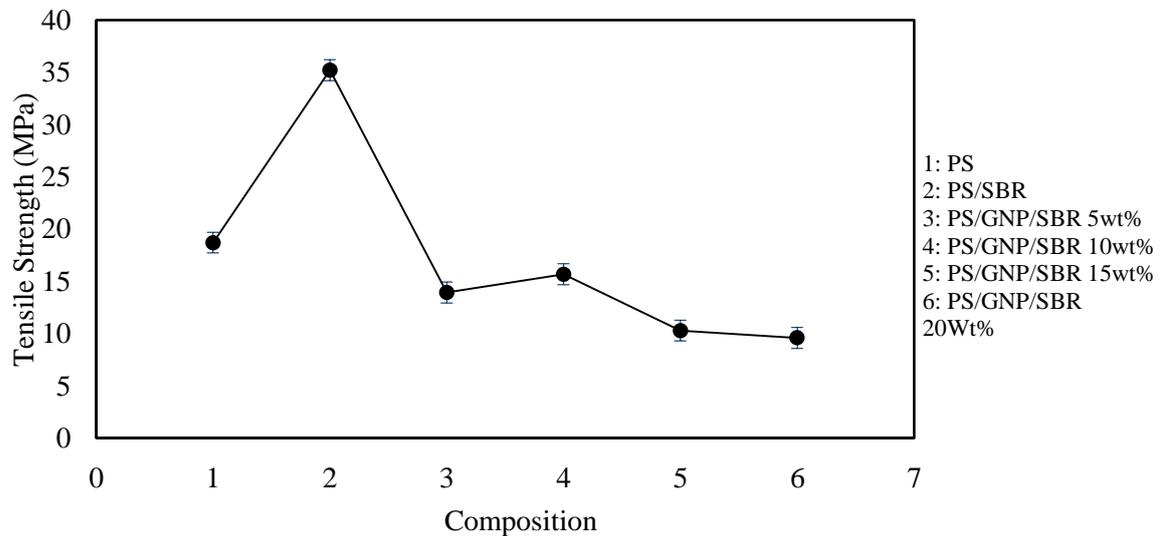
**Figure 2.** Tensile strength of SBR toughened PS/GNP nanocomposites at various contents of SBR.
