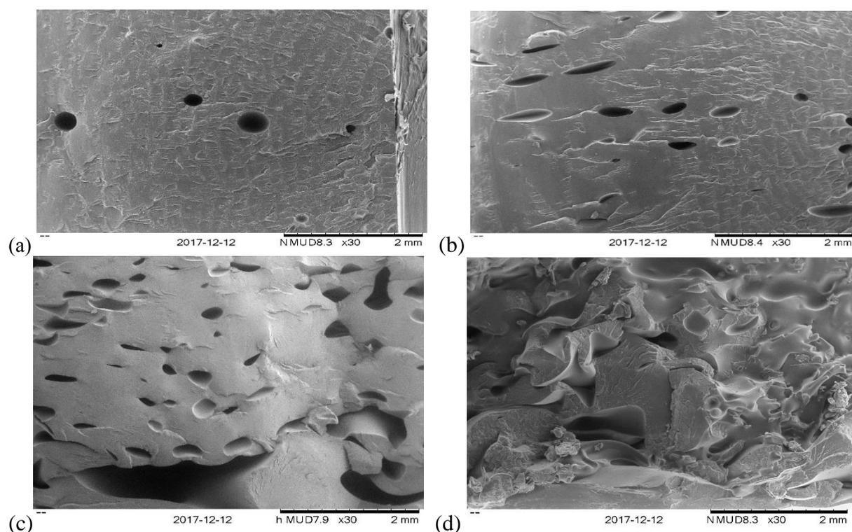
**Figure 1.** (a) Morphology Structure of PS/GNP (b) Morphology Structure of PS/SBR (c) Morphology Structure of PS/GNP with 5wt% SBR (d) Morphology Structure of PS/GNP with 20wt% SBR.
