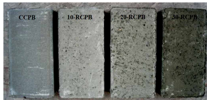
Figure 9. Rubberized concrete paving blocks Source: Ling (2011)
