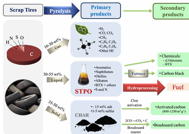
Figure 2. Primary and secondary products of waste tyre rubber Source: Akhil et al. (2018)
