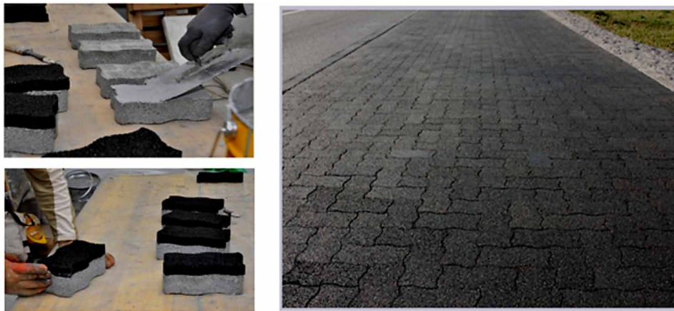
Figure 13. Poro-elastic block pavement made of PERS glued on concrete blocks and test track in Nova Gorica, Slovenia Source: Sandberg and Karman (2015)
