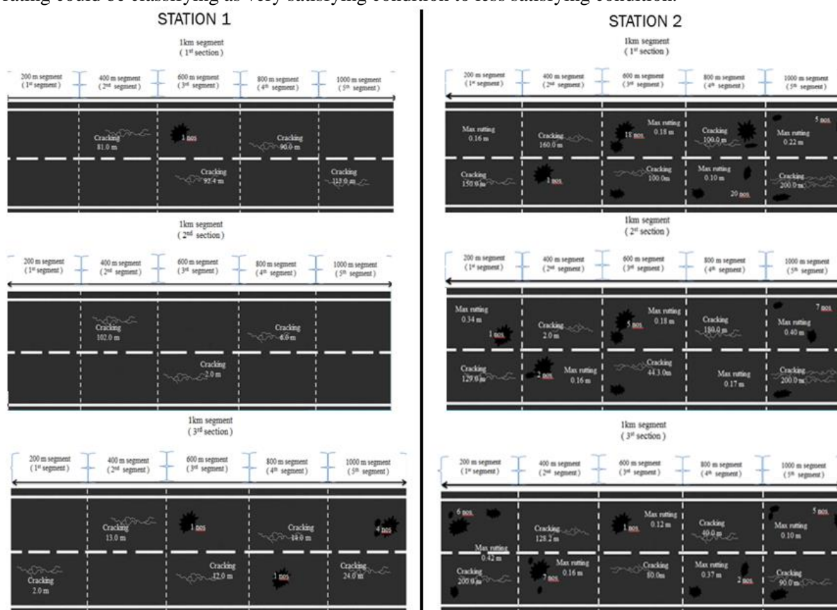
Figure 1: Illustration on Pavement Damages at Station 1 and Station 2
