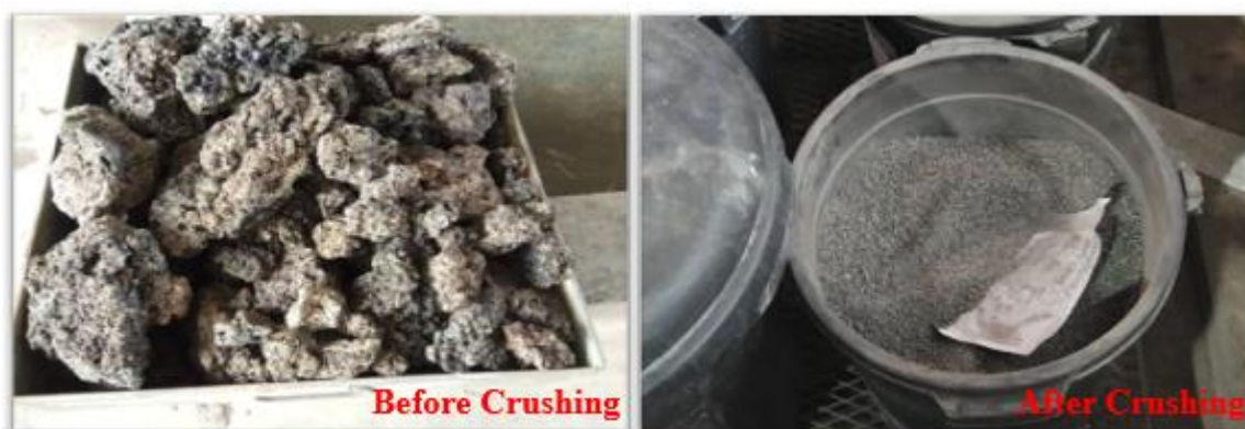
Figure 2: Palm oil clinker before and after crushing process
