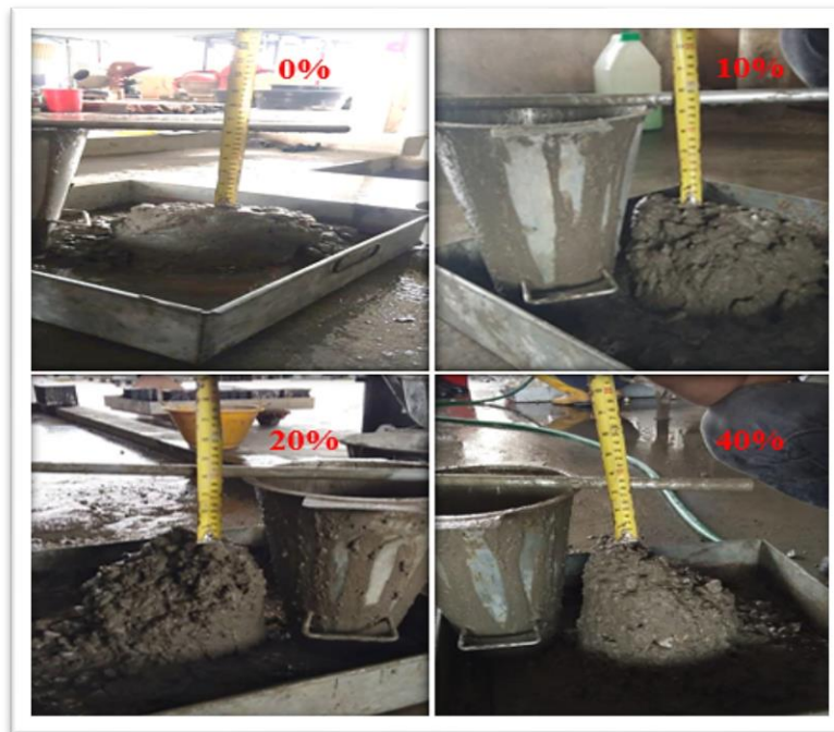
Figure 4: Effect of clinker on slump of concrete mix
