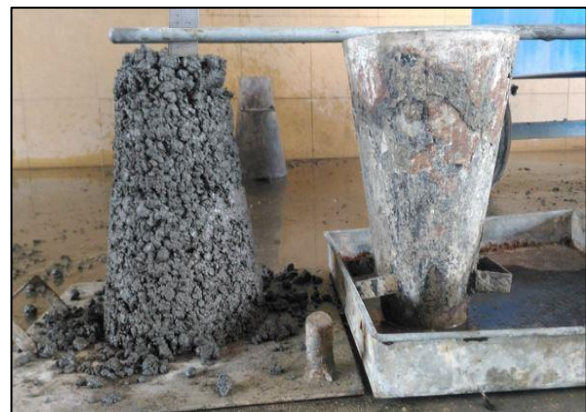
Figure 5. Slump of mix with 15% UPOFA
