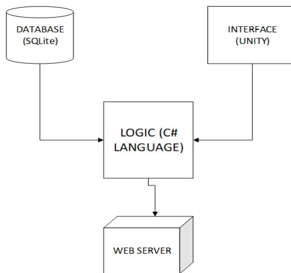
Figure 3.3 Software Architecture of the Application
