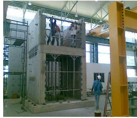
**Figure 2.** Construction of single bay double-storey house in the laboratory.
