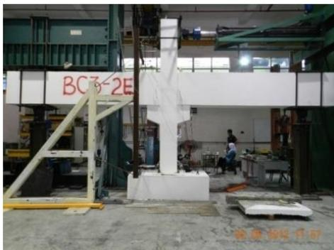
**Figure 3.** Super-assembly of precast beam-column joint is ready for testing
