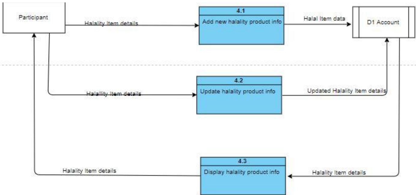
Figure 3.9: Data Flow Diagram Level 1 (Process 4.0 - Manage Halality Product Info)
