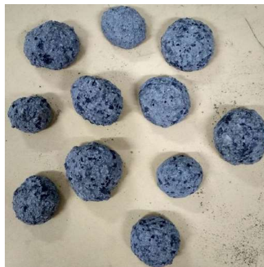
Fig. 1. Photo of manufactured electrically conductive aggregate
