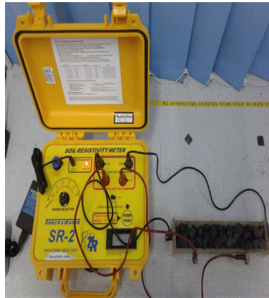
Fig. 2. Tinker & Rasor resistivity meter with soilbox attachment
