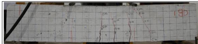
Figure 4. Crack pattern of CB
