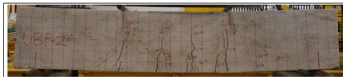
Figure 5. Crack pattern of VUSB
