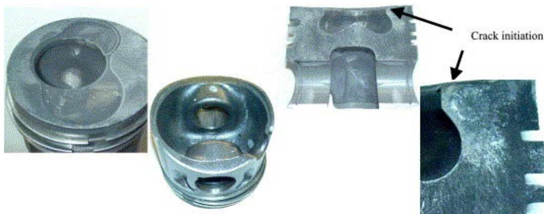
Figure 2.3: Diesel engine piston (with cooling gallery) with a crack from one side of the pin hole to the head [14]
