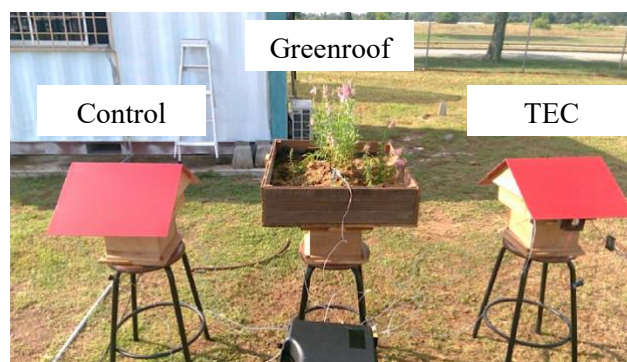
Figure 5: Overall setup, with thermocouples measuring temperatures inside honey cassette and brood cell compartment of each hives, connected to a temperature data logger
