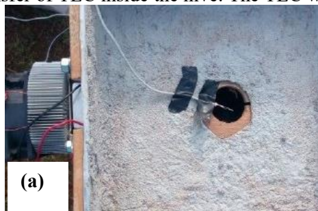
TEC fitted at the side of honey cassette, hot side coupled with a fan and the cold side attached to aluminium sheet inside honey cassette
