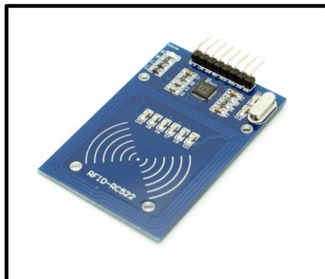
Figure 3.8 MIFAIR RC522 RFID Reader
