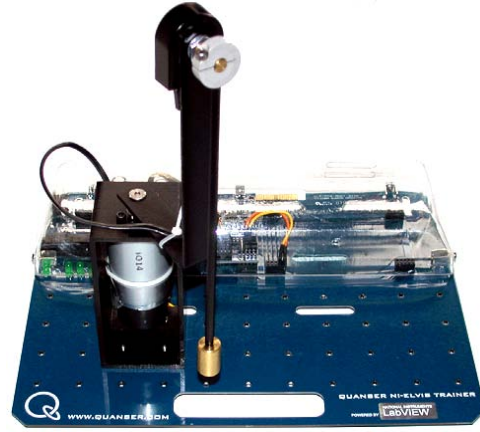
Fig. 2: Lab-scale rotary crane system
