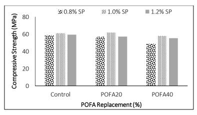
Fig. 4. The effect of superplasticizer content towards compressive strength of POC LWAC with POFA.
