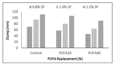
Fig. 3. The effect of superplasticizer content towards workability of POC LWAC with POFA.
