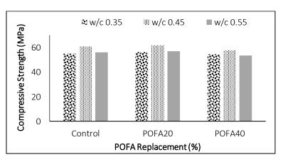
Fig. 2. The effect of water-cement ratio towards compressive strength of POC LWAC with POFA.
