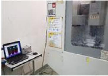
**Fig. 2 – Machining and cutting force measurement on HAAS CNC milling machine**
