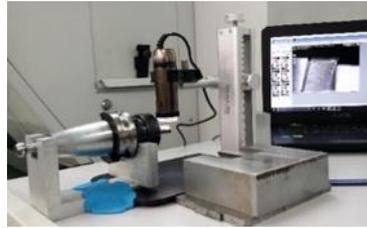
**Fig. 5 - Tool maker’s microscope**
