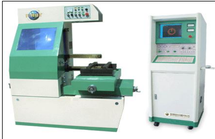
Figure 2.1 : Wire Electro Discharge Machining [14]
